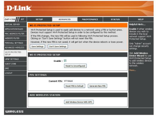
Generate New Create a random number that is a valid PIN. This becomes the router's PIN. You can then copy this PIN to the user interface PIN: of the registrar.
